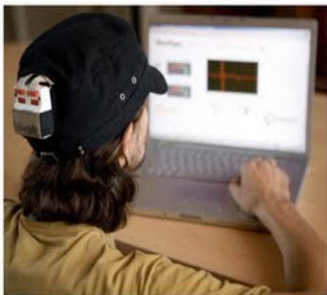
Fig. 1: ENOBIO sensor embedded in a cap. We can see the 4 channel inputs (red pins). In the picture, only two channels are plugged. The data are transmitted wirelessly to the laptop.
